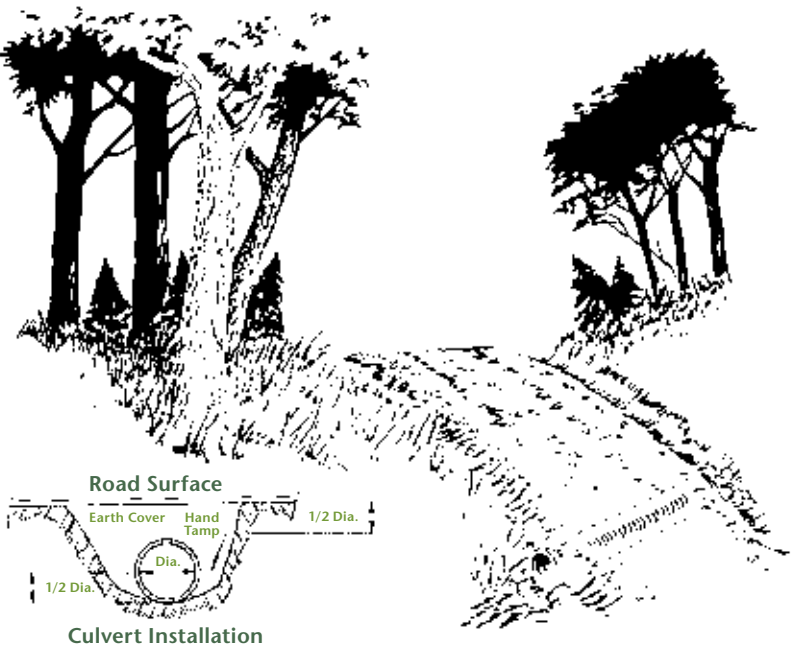
Figure 3. Installing a Culvert Pipe
